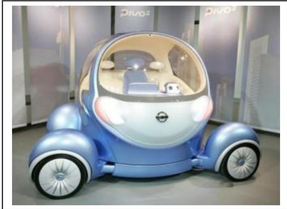
*Pivo 2 employs 'by-wire' technologies for braking and steering and features a 360 degree turning cabin and 90 degree turning wheels that makes reversing a thing of the past. In addition to advancements on this radical rotational design, the second generation Pivo uses a Robotic Agent to create a unique owner-vehicle relationship that is a kin to that of a friend.*
